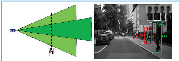
AEB System: Road scene analysis and recognition of Vulnerable Road Users
