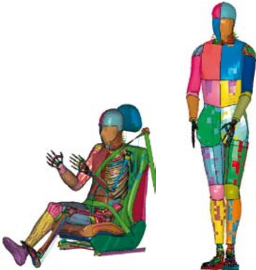
*Figure 8: Visualisation of biofidelic human body modeling used for simulation of advanced protection systems*
