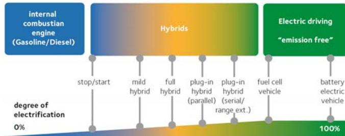
Figure 5: Electrification of the powertrain
