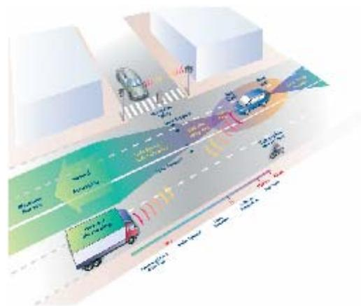
Figure 6: Cooperative systems – Vehicle-to-vehicle and vehicle-to-infrastructure communication
