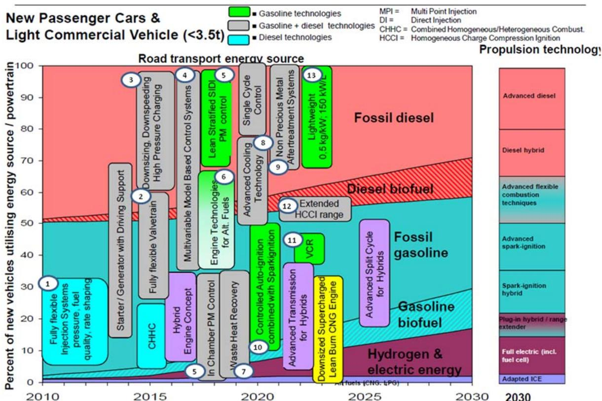
Figure 4: Main technology trends and the vision of share of engines in Europe (EUCAR Working Group Powertrain 2010)
